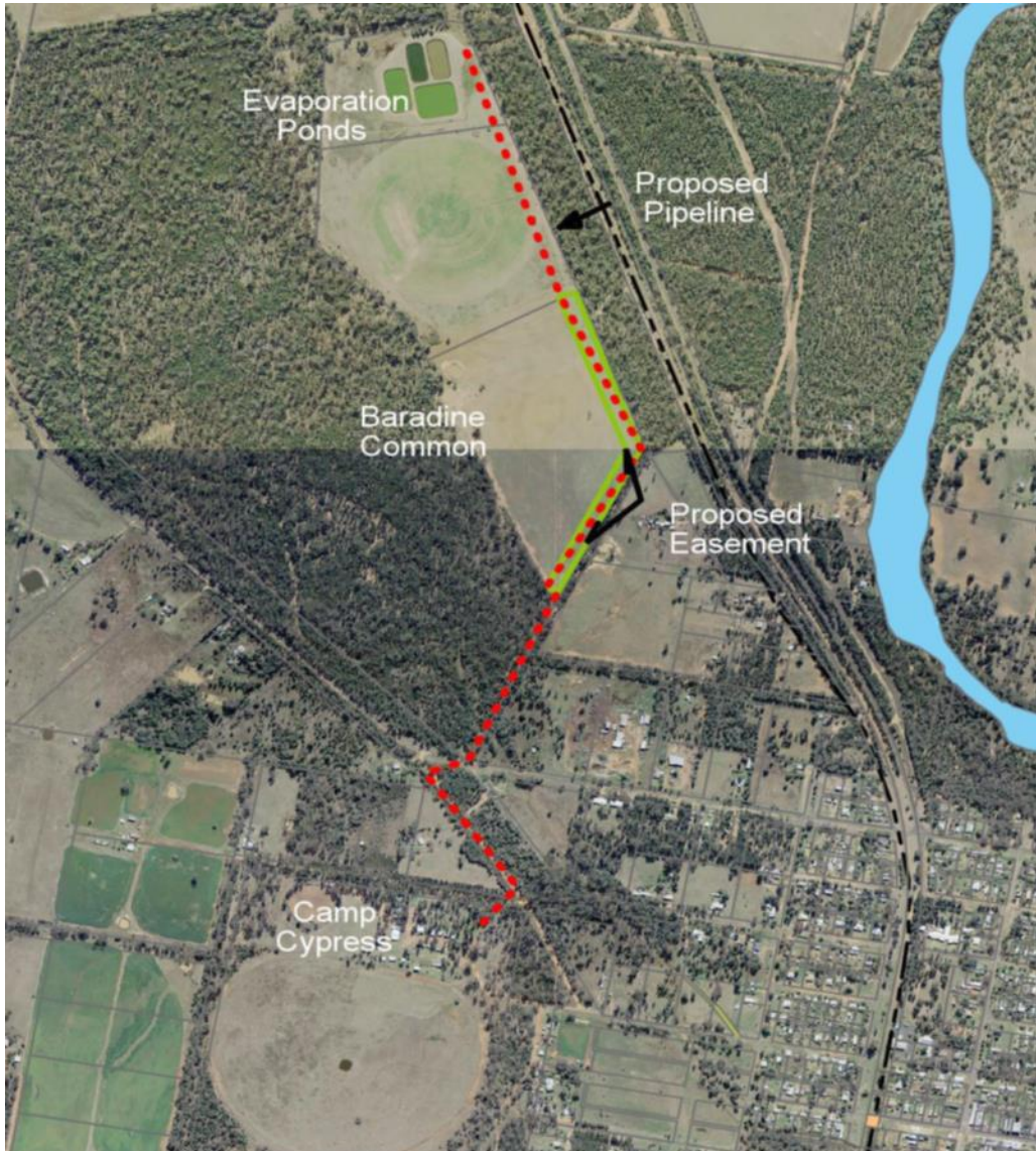
Figure 3-2: Location of Proposed Sewer Pipeline Connecting Camp Cypress to the Baradine STP
